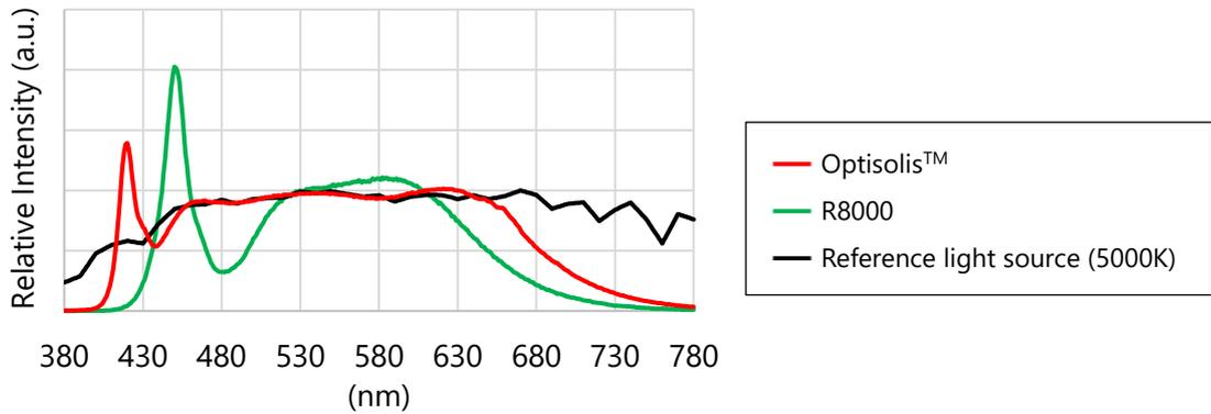
Figure 3. Example wavelength of the Optisolis™ LED<sup>4</sup>
