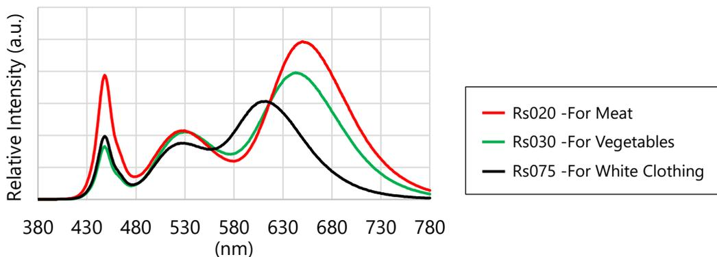
Figure 4. Example wavelengths for the special CRI ranks<sup>5</sup>
