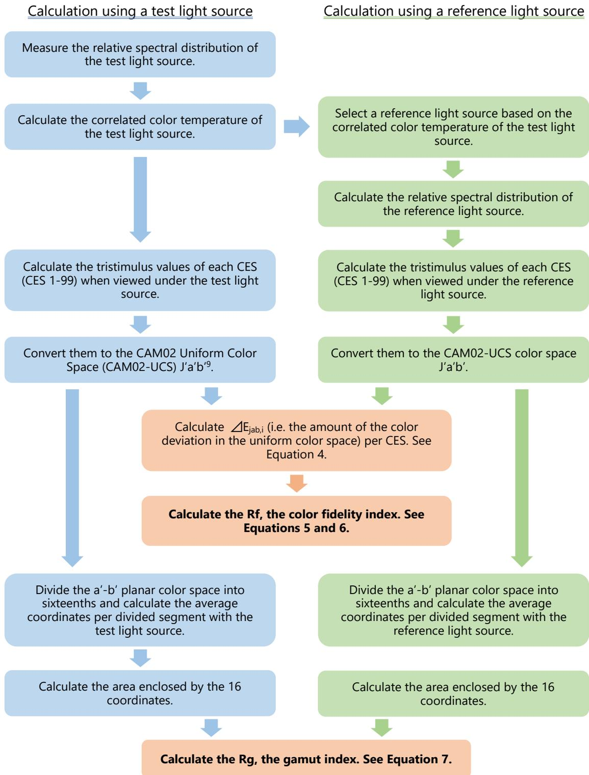
Figure 9. How to determine Rf and Rg values
