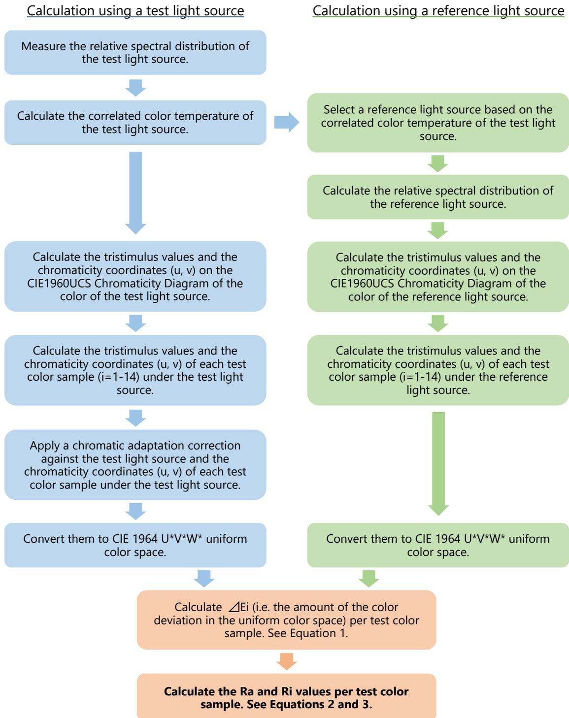
Figure 5. How to determine Ra and Ri values
